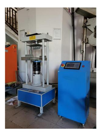
Bending Test Machine is used for bending strength test with midpoint loading in accordance with TS EN 12390-5, ASTM C78 and ASTM C293 standards on 100x100x400-500 mm and 150x150x600-750 mm sized specimens.
